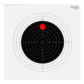
If the shot is high of the center then turn the "elevation" **UP** (Counterclockwise)
