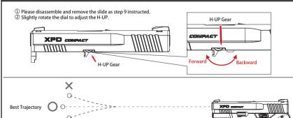
H-up Adjustment: Make sure the trajectory of the BB pellets to be straight. When the BB pellet flies up: Rotate the dial forward to lower the trajectory. When the BB pellet falls down: Rotate the dial backward to raise the trajectory.
