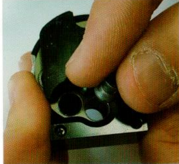
After seating first pellet properly , turn mag so pellet appears in center hole and insert next pellet. Repeat like this
