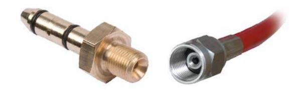
You should tighten finger tight + approx 1/2 - 3/4 of a turn. This is usually sufficient for all applications encountered. If the connection leaks on initial pressurization, you can tighten by further 1/4 turns until a seal is achieved.
