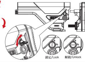
齒輪箱拆解 Disassemble Gearbox
