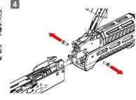
將槍管座螺絲卸下,並將槍身前段往前抽出。 Remove the barrel mount screws, and then pull the front assembly forward to remove.
