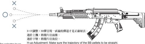
H-up Adjustment: Make sure the trajectory of the BB pellets to be straight. When the BB pellet flies up: Push the H-UP lever forward to lower the trajectory. When the BB pellet falls down: Push the H-UP lever backward to raise the trajectory.
