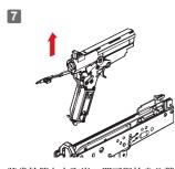
將齒輪箱向上取出,即可與槍身分離。 Remove the Ergo grip and the fire selector Remove the gearbox upward to separate it from the receiver.
