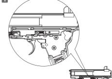
Install Gearbox into Receiver.
