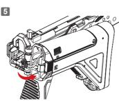
將槍托摺疊後,把線材抽出槍托。 Fold the stock and then and unplug
