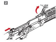
壓下機匣蓋開關後,將機匣蓋向上打開固 定在前。(需確實向前固定避免落下夾傷) Press the upper receiver catch to open the remove the charging handle set. upper receiver cover and keep it opening in the front. (Avoid the upper receiver falling from hands clipping)
