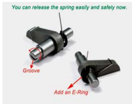
Redesigned Anti-reversal latch
